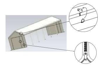
5. Lift the other side of the roof section and attach the legs.
