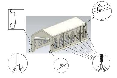
7. Attach the canopy to every bar framework using the elastic bungee toggle straps, Velcro attached to roof canopy and frame tieing the structure together providing wind proof enclosure
