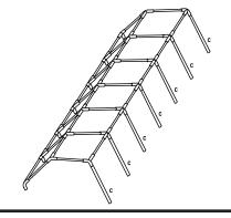
3. Using the required number of people, lift one side of the Gala Tent™ and insert the legs. Ensure that the holes in the poles are placed towards the bottom as the leg cover clips to these.
