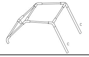
3. Using the required number of people, lift one side of the Gala Tent™ and insert the legs. Ensure that the holes in the poles are placed towards the bottom as the leg cover clips to these.
