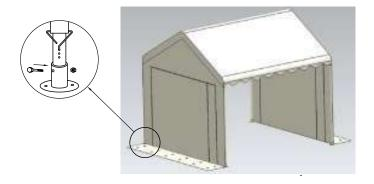
6. Attach the sidewalls to every bar framework using the elastic bungee toggle straps, Velcro attached to leg poles, zips or dutch lacing, tie the side walls together providing wind proof enclosure
