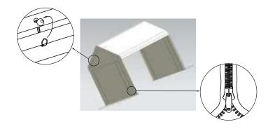
5. Lift the other side of the roof section and attach the legs. Attach the pedestal feet to the bottom of all the legs using the nuts and bolts provided.
