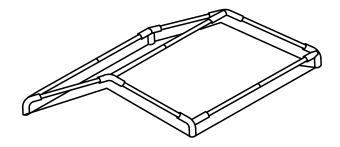
3. Using the required number of people, lift one side of the Gala Tent™ and insert the legs. Ensure that the holes in the poles are placed towards the bottom as the leg cover clips to these.
