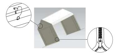
5. Lift the other side of the roof section and attach the legs.
