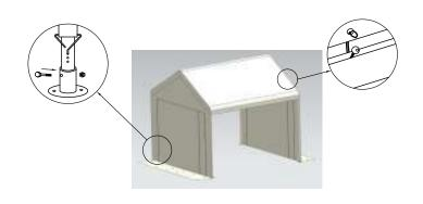
6. Attach the sidewalls to every bar framework using the elastic bungee toggle straps, Velcro attached to leg poles, zips or dutch lacing, tie the side walls together providing wind proof enclosure
