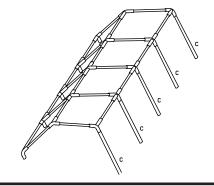
3. Using the required number of people, lift one side of the Gala Tent™ and insert the legs. Ensure that the holes in the poles are placed towards the bottom as the leg cover clips to these.
