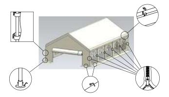
7. Attach the canopy to every bar framework using the elastic bungee toggle straps, Velcro attached to roof canopy and frame tieing the structure together providing wind proof enclosure
