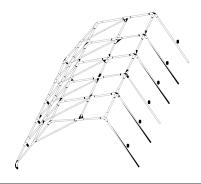
3. Using the required number of people, lift one side of the Gala Tent™ and insert the legs. Ensure that the holes in the poles are placed towards the bottom as the leg cover clips to these.
