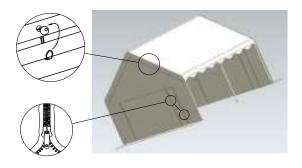
5. Lift the other side of the roof section and attach the legs.
