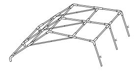
3. Using the required number of people, lift one side of the Gala Tent™ and insert the legs. Ensure that the holes in the poles are placed towards the bottom as the leg cover clips to these.
