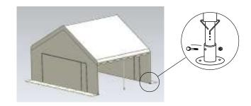
6. Attach the sidewalls to every bar framework using the elastic bungee toggle straps, Velcro attached to leg poles, zips or dutch lacing, tie the side walls together providing wind proof enclosure
