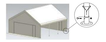
6. Attach the sidewalls to every bar framework using the elastic bungee toggle straps, Velcro attached to leg poles, zips or dutch lacing, tie the side walls together providing wind proof enclosure
