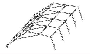
3. Using the required number of people, lift one side of the Gala Tent™ and insert the legs. Ensure that the holes in the poles are placed towards the bottom as the leg cover clips to these.
