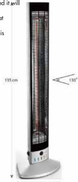
Dimensions: L37xW48xH143cm Weight: 18.1kg Projection angle: 130° at 3.5m distance Heating Power: 208 – 240V 50Hz/60Hz 1800W
