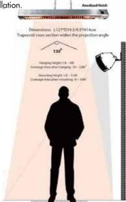
Dimensions: L 127xD19.5/9.5xH14cm Projection angle: 130° Hanging Height: 1.8m - 4m Coverage area when hanging: 10m - 22m squared Mounting Height: 1.8m - 3.5m Coverage area when mounted: 8m - 16m squared Heating Power: 208 - 240V 50Hz/60Hz 2800W Safe Touch Safe Touch Safe Touch Safe Touch DIM Carbon <u>3 Year</u>
