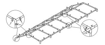
2. Lay the roof cover over the frame and attach using the elastic bungee toggle straps provided.
