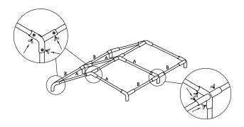
2. Lay the roof cover over the frame and attach using the elastic bungee toggle straps provided.
