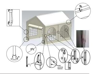
7. Attach the canopy to every bar framework using the elastic bungee toggle straps, Velcro attached to roof canopy and frame tieing the structure together providing wind proof enclosure
