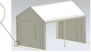
6. Attach the sidewalls to every bar framework using the elastic bungee toggle straps, Velcro attached to leg poles, zips or dutch lacing, tie the side walls together providing wind proof enclosure
