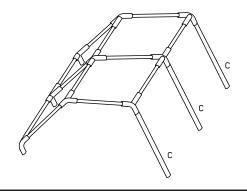
3. Using the required number of people, lift one side of the Gala Tent™ and insert the legs. Ensure that the holes in the poles are placed towards the bottom as the leg cover clips to these.
