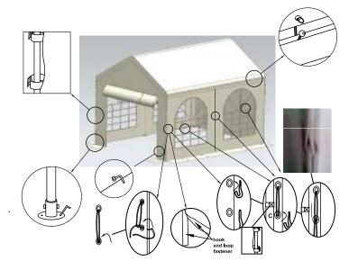
7. Attach the canopy to every bar framework using the elastic bungee toggle straps, Velcro attached to roof canopy and frame tieing the structure together providing wind proof enclosure
