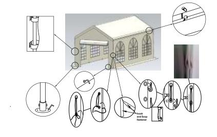
7. Attach the canopy to every bar framework using the elastic bungee toggle straps, Velcro attached to roof canopy and frame tieing the structure together providing wind proof enclosure
