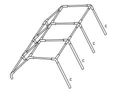
3. Using the required number of people, lift one side of the Gala Tent™ and insert the legs. Ensure that the holes in the poles are placed towards the bottom as the leg cover clips to these.
