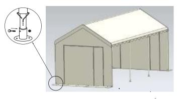
6. Attach the sidewalls to every bar framework using the elastic bungee toggle straps, Velcro attached to leg poles, zips or dutch lacing, tie the side walls together providing wind proof enclosure
