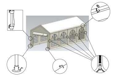
7. Attach the canopy to every bar framework using the elastic bungee toggle straps, Velcro attached to roof canopy and frame tieing the structure together providing wind proof enclosure
