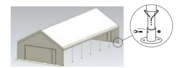
6. Attach the sidewalls to every bar framework using the elastic bungee toggle straps, Velcro attached to leg poles, zips or dutch lacing, tie the side walls together providing wind proof enclosure
