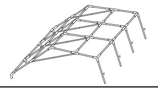
3. Using the required number of people, lift one side of the Gala Tent™ and insert the legs. Ensure that the holes in the poles are placed towards the bottom as the leg cover clips to these.
