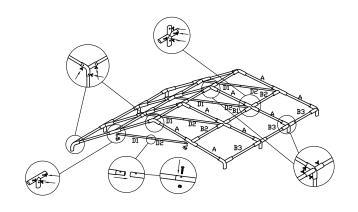
2. Lay the roof cover over the frame and attach using the elastic bungee toggle straps provided.
