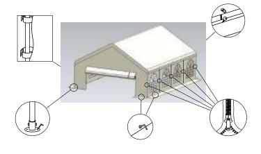
7. Attach the canopy to every bar framework using the elastic bungee toggle straps, Velcro attached to roof canopy and frame tieing the structure together providing wind proof enclosure
