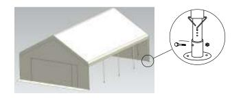
6. Attach the sidewalls to every bar framework using the elastic bungee toggle straps, Velcro attached to leg poles, zips or dutch lacing, tie the side walls together providing wind proof enclosure
